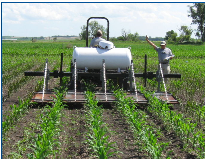
Figure 4: Four-row flame weeding system developed by the University of Nebraska, Lincoln and Agricultural Flaming Innovations, Nebraska
