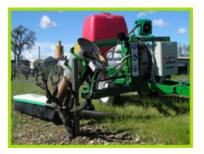
During the presentation, *Steam Weed Control*, *A Proven Propane Solution*, Jacobs said, "*The Stinger*, which is currently being tested at Cal Poly, San Luis Obispo, is a cutting-edge agricultural tool that utilizes propane and water to generate steam to control weeds in orchards and vineyards." Developed in Australia by D.J. Batchen Pty. Ltd., the Batchen *Stinger* allows farmers to implement an environmentally friendly
